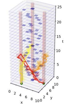
A 3D plot showing a search tree for three robots. The vertical axis is time (t) from 0 to 25. The horizontal axes are position (x) from 0 to 10 and orientation (y) from 0 to 10. The tree is a complex structure of colored nodes (blue, red, yellow) and connecting edges, representing a search space with obstacles. | <a href="#">3b t3 v.mov</a> | 1286 | 1132 |
