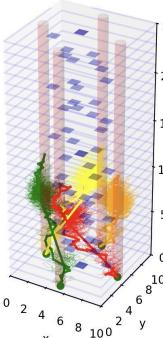
A 3D plot showing a search tree for four robots in trial 1. The axes are time (t) 0-25, position (x) 0-10, and orientation (y) 0-10. The tree is more complex than the 3-robot case, with many more nodes and a more intricate branching structure. | <a href="#">4 bots, 2 ...</a> | 5372                              | 4010                    |
